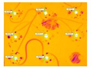
Fig. 10. A study of temperature distributions on LEDs cases using infrared thermography; ambient temperature is 35 ° C.
