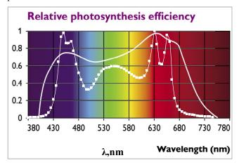
Fig. 8. SPD of LED module (three neutral white, one blue, one royal blue, one red and one deep red LEDs, which spectrum is shown in Fig. 6, curve 2), compared to the relative photosynthesis efficiency [8].
