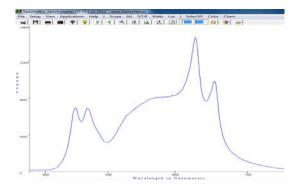
Fig. 5. LEDs' spectral characteristics: three warm white LEDs at 350mA; royal blue (XPCROY), blue (XPCBLU), red (XPCRED) and deep red (HPL) at 200mA.
