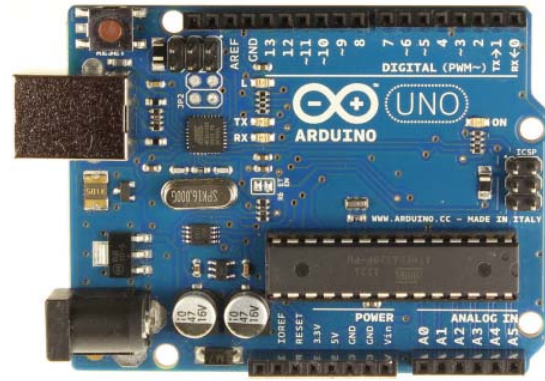
Fig. 4. Arduino microcontroller board [3]
