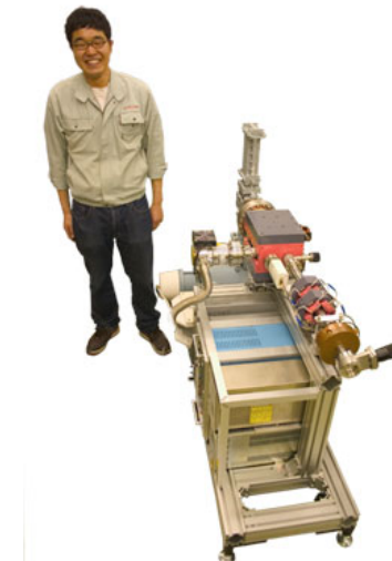
Fig. 5. Photo of the smallest model of MIRRORCLE - for E_{el} = 1 MeV
