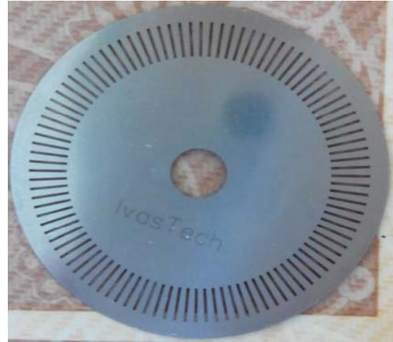
Fig. 2. Disc used in the motion tracking sensor
