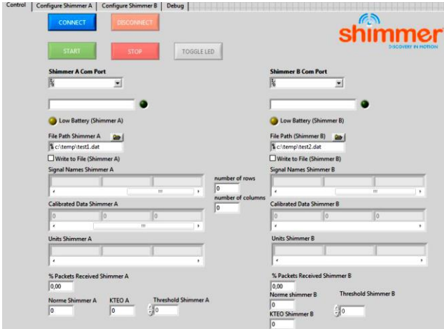
Fig. 2. A screenshot of the adapted front-end for reading and modifying sensor nodes
