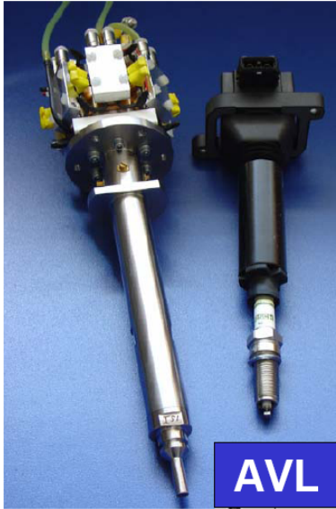
Fig. 3. Different laser sparkplugs developed worldwide: Concept Carynthian Tech Research Villach / AVL Graz, Austria, based on transversally diode-pumped Q-switched Nd:YAG laser [20].
