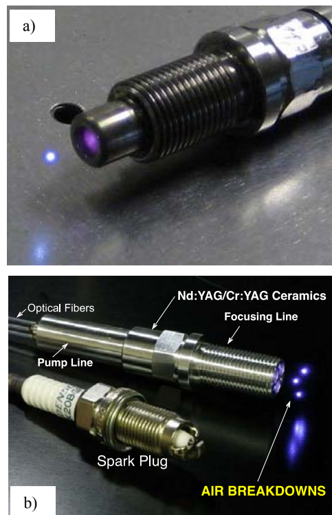
Fig. 2. Different laser sparkplugs developed by pioneering research groups: a) Laser Ignition Group Vienna University of Technology, Vienna, Austria [8], b) Institute of Molecular Science, Okazaki, Japan [19], both longitudinally fiber-coupled diode pumped Q-switched Nd:YAG lasers.
